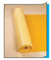
Unroll the Lok-Lift in the same direction as the carpet is to be installed, with the yellow plastic liner on top
